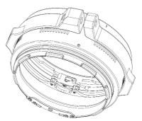
1. Mount the mounting bracket for trim weights on an extension ring.
