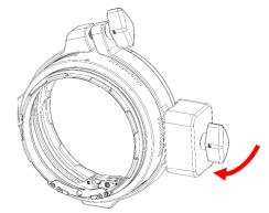
4. Tightly fasten the trim weight by thumb screw as shown.
