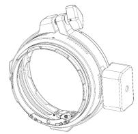
3. Mount a trim weight onto screw hole of mounting bracket.
