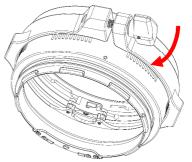
2. Securely fasten it by thumb screw as shown.
